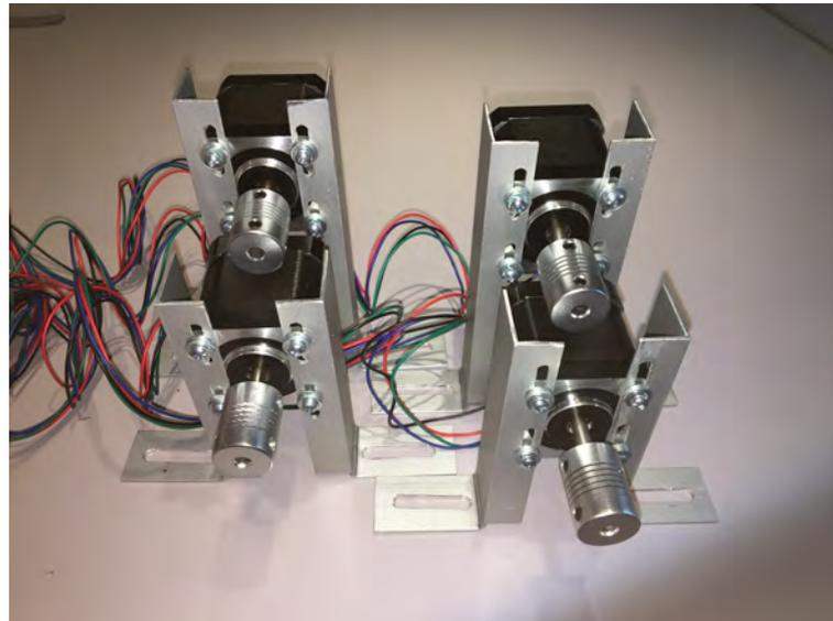
Figure 4.13: *Mechanical setup of the steppers.*
