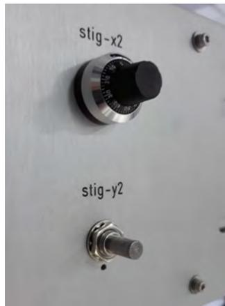
Figure 4.11: *Potentiometer knob with and without cover.*
