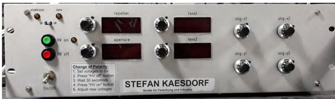
Figure 4.10: *Front panel of IMT12 showing the control potentiometers of repeller, extractor aka aperture, lens1 and lens2.*
