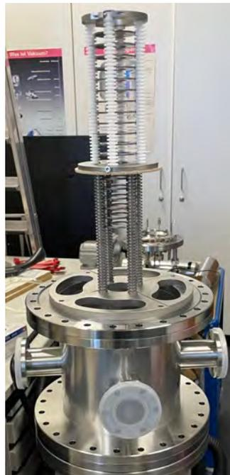
Figure 4.23: *The GIM's electrodes manufactured by the MPQ workshop.*
