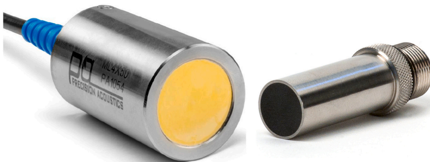
Fig. 4. Immersion transducers used in our ionoacoustic setups: (left) Circular plane piston hydrophone ML4X50 based on gold coated PVDF foils, active diameter 23 mm (Precision Acoustics, Dorchester, UK). (right) Focused PZT transducer, active diameter 13 mm (Videoscan, Olympus, Germany).
