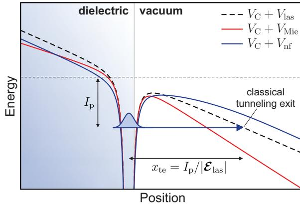
**Figure 8.** Schematic representation of tunneling from the surface of a dielectric. The dashed black curve reflects the effective potential for the atomic case (Coulomb + Laser). Solid red and blue curves represent the effective potentials when considering the enhanced linear (Mie) near-field and the full near-field for an atom located near the surface of a dielectric, respectively. From [45].
