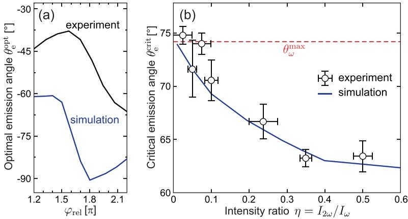
**Figure 22.** (a) Relative phase-dependent optimal emission angles for downward emission obtained from experiment (black) and simulation (blue) with 300 nm SiO<sub>2</sub> nanospheres at  $\eta = 0.5$  (cf. black curves in Figure 21(d,g)). (b) Intensity ratio-dependent critical emission angles for upward emission obtained from measurement (circles) and SMM simulations (solid blue curve) with 300 nm SiO<sub>2</sub> nanospheres. Adapted from [51] under Creative Commons Attribution 3.0 licence.
