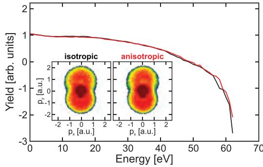
**Figure 13.** Impact of anisotropic elastic collisions on the electron emission from  $d = 100$  nm  $\text{SiO}_2$  nanoparticles under 4 fs NIR few-cycle pulses ( $\lambda = 720$  nm,  $I = 3 \times 10^{13}$  W/cm $^2$ ,  $\varphi_{ce} = 0$ ). From [45].
