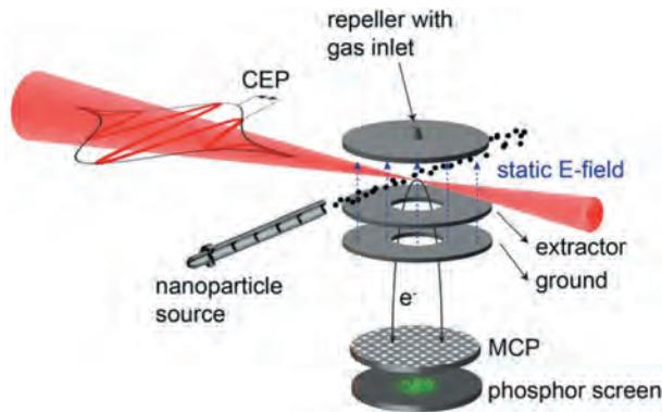
**Figure 4.** Schematic representation of VMI of strong-field induced ionization processes in isolated nanoparticles. Courtesy of Philipp Rupp.
