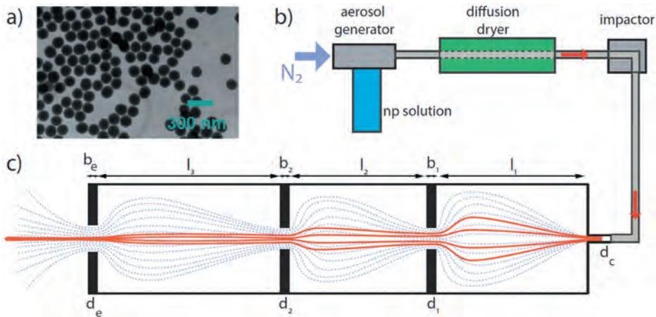
**Figure 3.** (a) TEM image of  $SiO_2$  nanospheres with a diameter of 147 nm. (b) Flow diagram for the generation of the nanoparticle aerosol. (c) Working principle of an aerodynamic nanoparticle lens. The trajectories of gas molecules are schematically indicated by the blue dashed lines. The nanoparticle trajectories are shown in red. From [62].
