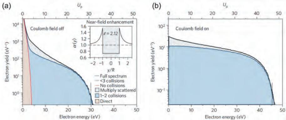
**Figure 12.** Impact of charge interaction on the electron emission from silica nanospheres (100 nm diameter) under intense few-cycle fields. **(a,b)** Simulated photoelectron energy spectra of electrons with different numbers of elastic collisions (as indicated) with charge interaction turned off (a) and on (b). The inset in (a) shows the spatial field enhancement profile along the laser fields polarization axis. From [40].
