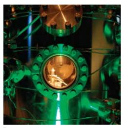
The attosecond-scale measurement scheme uses a commercial Ti:sapphire laser to deliver waveform-controlled few-cycle, 5 fs near-infrared (750 nm) laser pulses at a repetition rate of 4 kHz. The laser pulses produce isolated coincident 300-attosecond EUV pulses used for real-time observation of rapid electron motion inside atoms, molecules, and solids. (Courtesy of Max-Planck-Institut für Quantenoptik/Thorsten Naeser)
