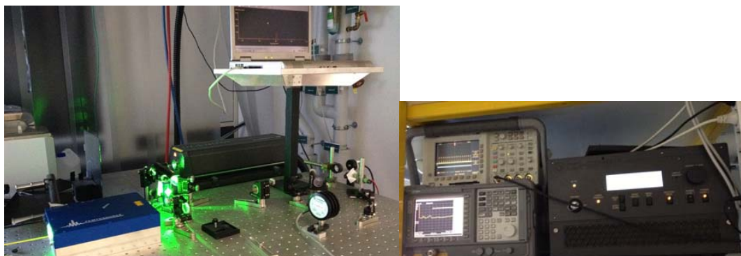
Fig.14. Left: Photo of the femtosecond Ti:Sa oscillator together with Verdi pump laser and the computer for detecting spectra and the pulse train. Right: Verdi power supply (right), spectrum analyzer for recording the beat signals at the harmonics of the laser repetition rates (left bottom) and oscilloscope to record the pulse train.
